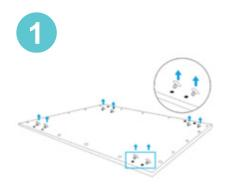
Fix the ceiling frame & fasten the clips into the ceiling where panel light is to be installed.
