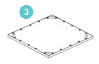
Hang the retaining rings on the hook, connect the power cord and then LED panel can be used.
